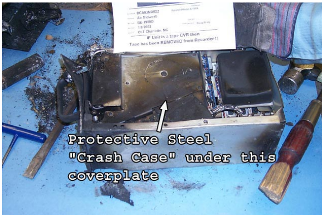
Figure 3 - Exterior Dustcover Removed
